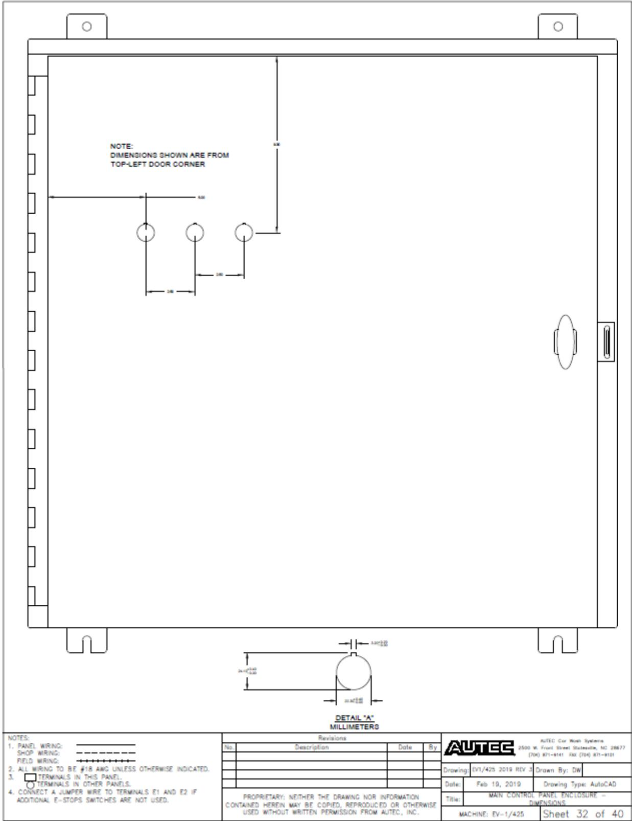
Fig 9-32 Main Control Enclosure – Dimensions
