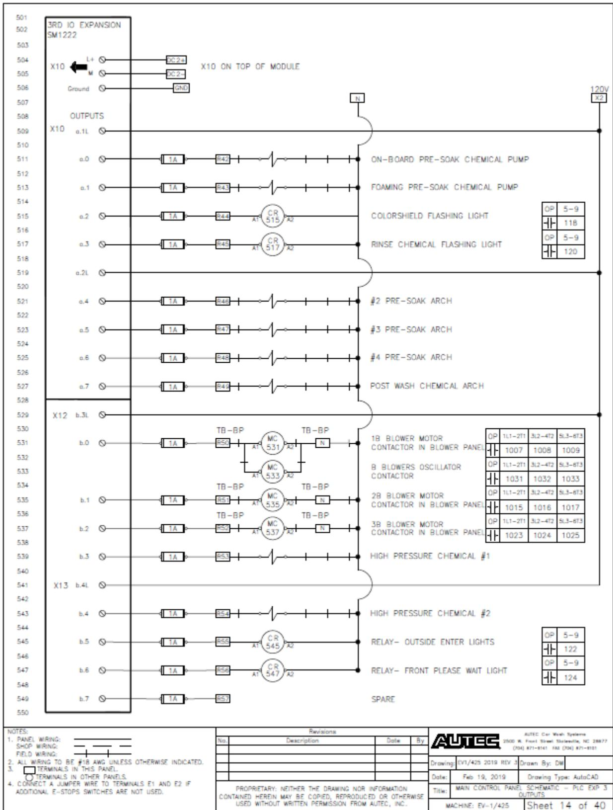
Fig 9-14 Main Control Panel Schematic – Mod 3 Outputs
