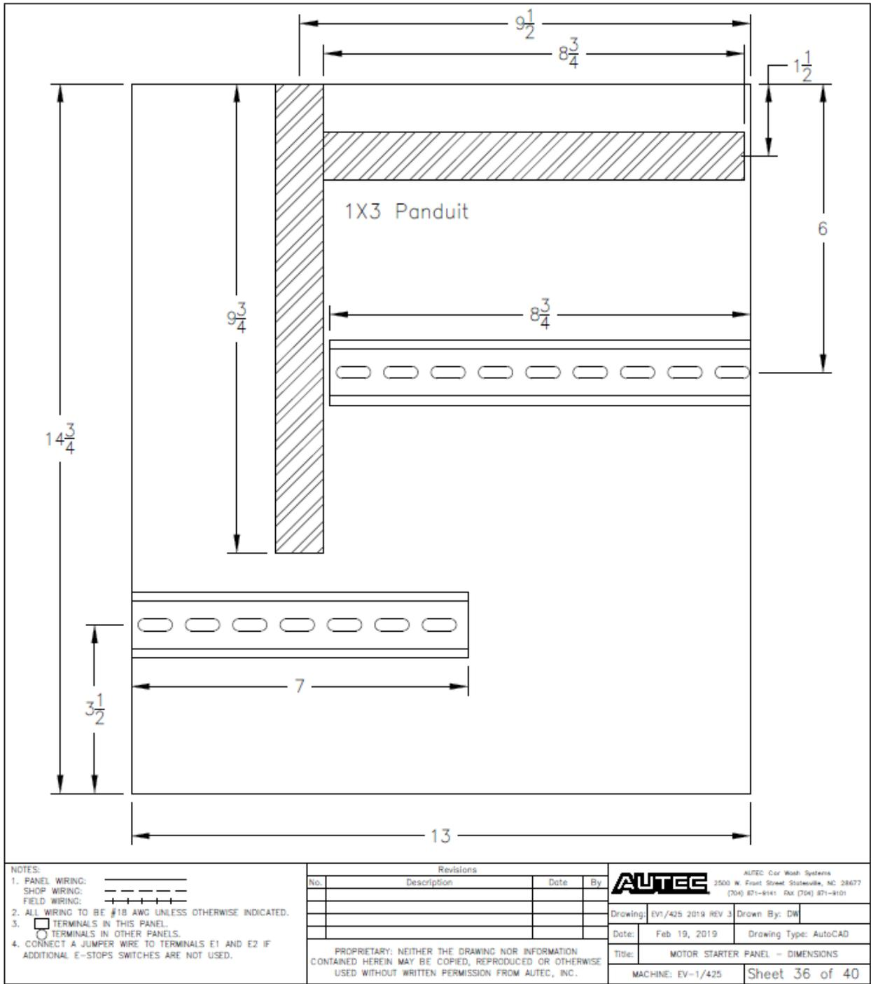
Fig 9-36 Motor Starter Panel – Dimensions
