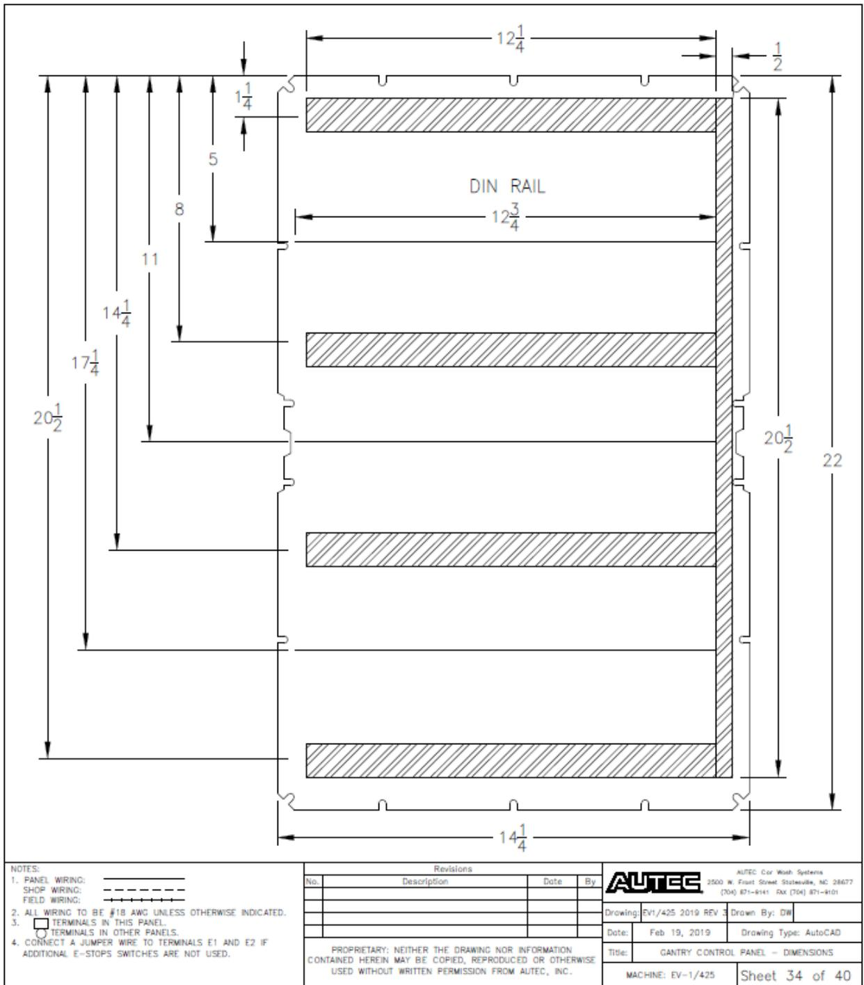
Fig 9-34 Gantry Control Panel – Dimensions
