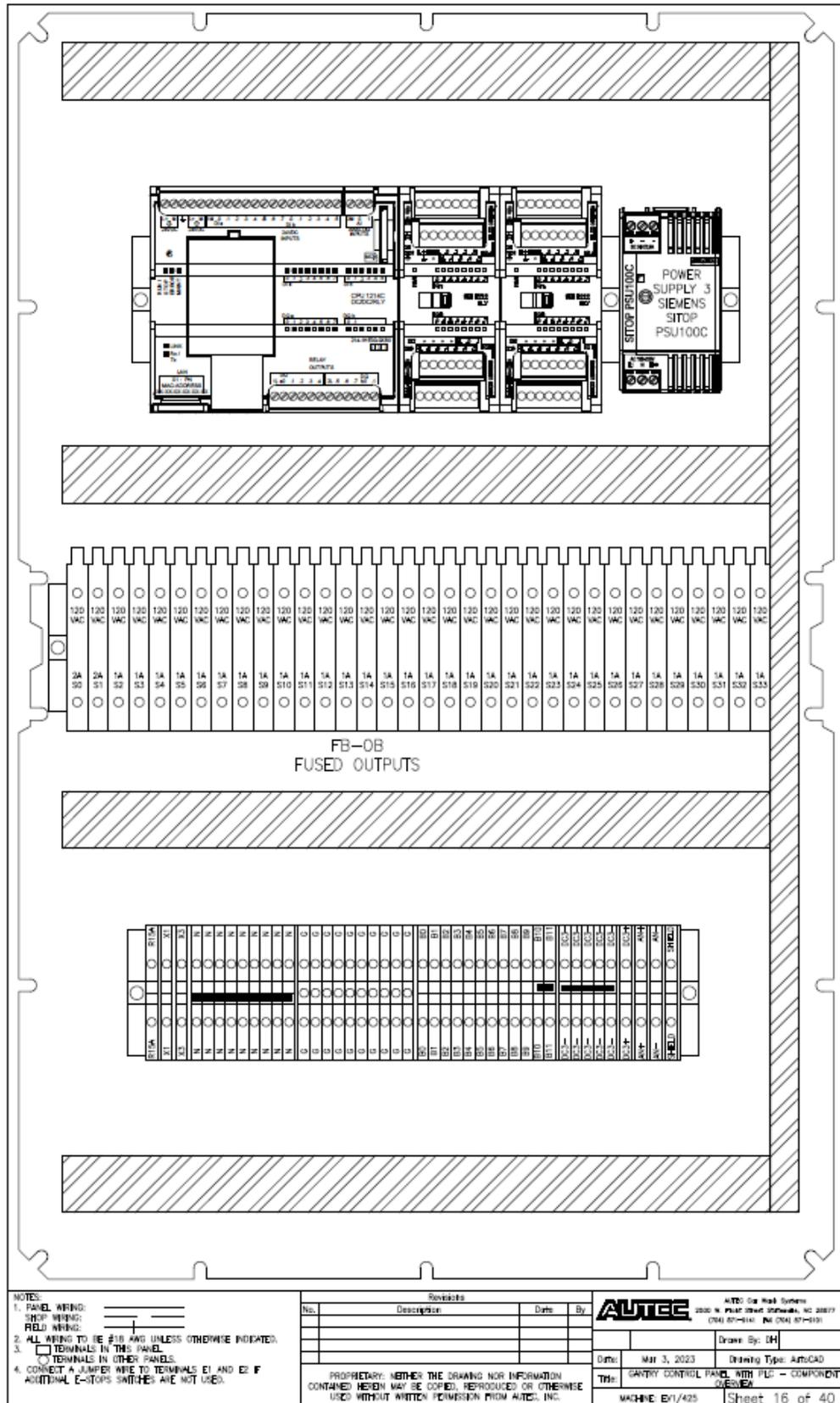
Fig 9-16 Gantry Control Panel – Component Layout
