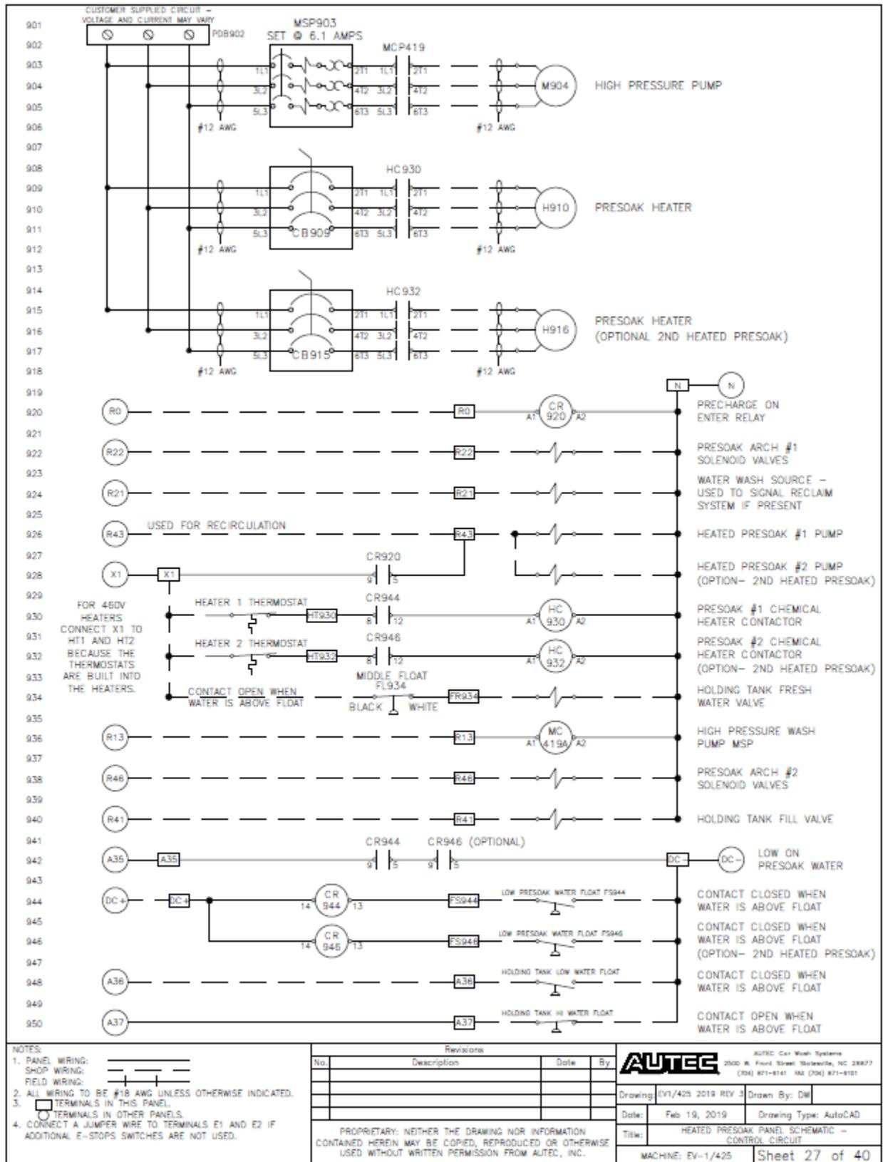
Fig 9-27 Heated Presoak Panel Schematic – Control Circuit
