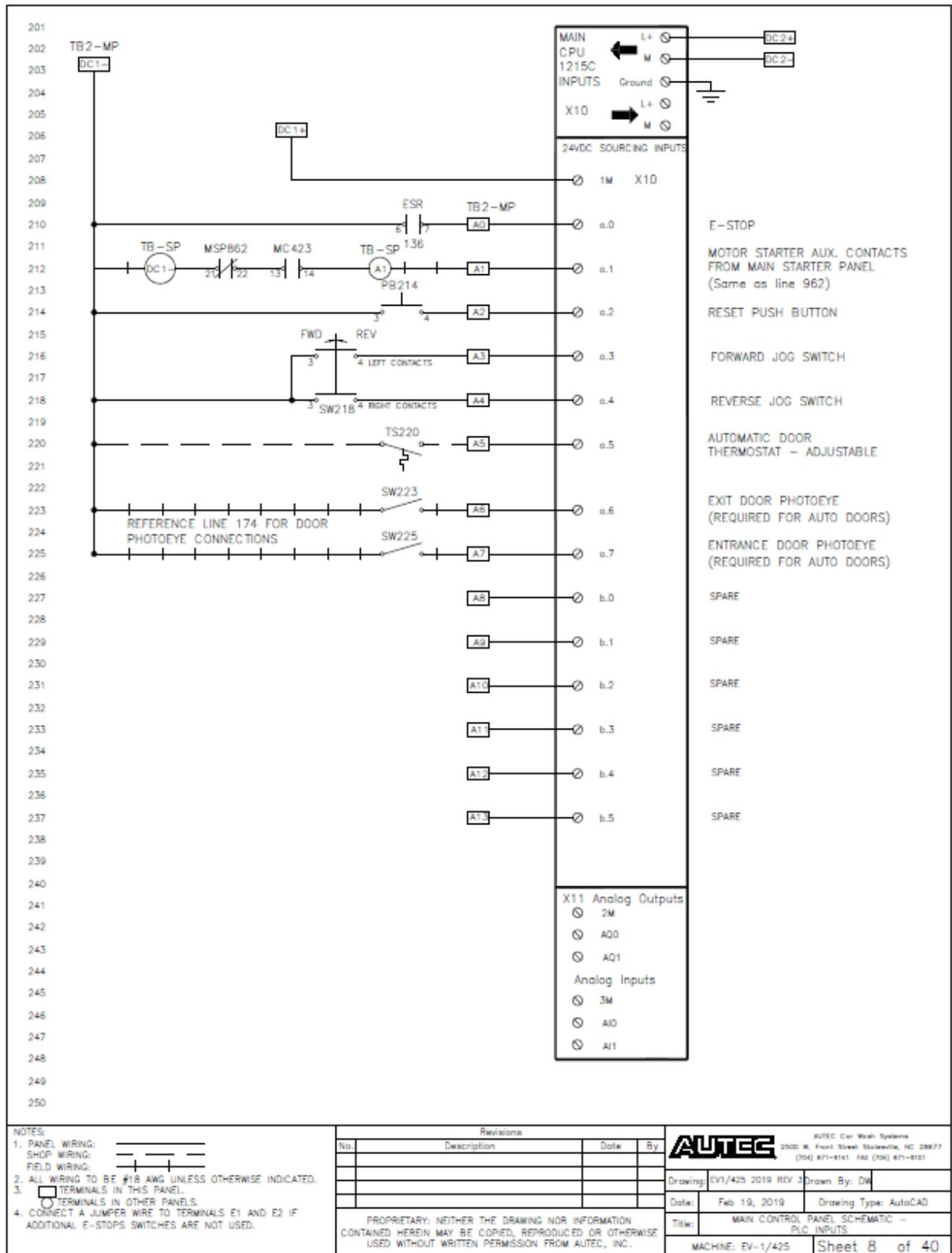
Fig 9-8 Main Control Panel Schematic – PLC Inputs
