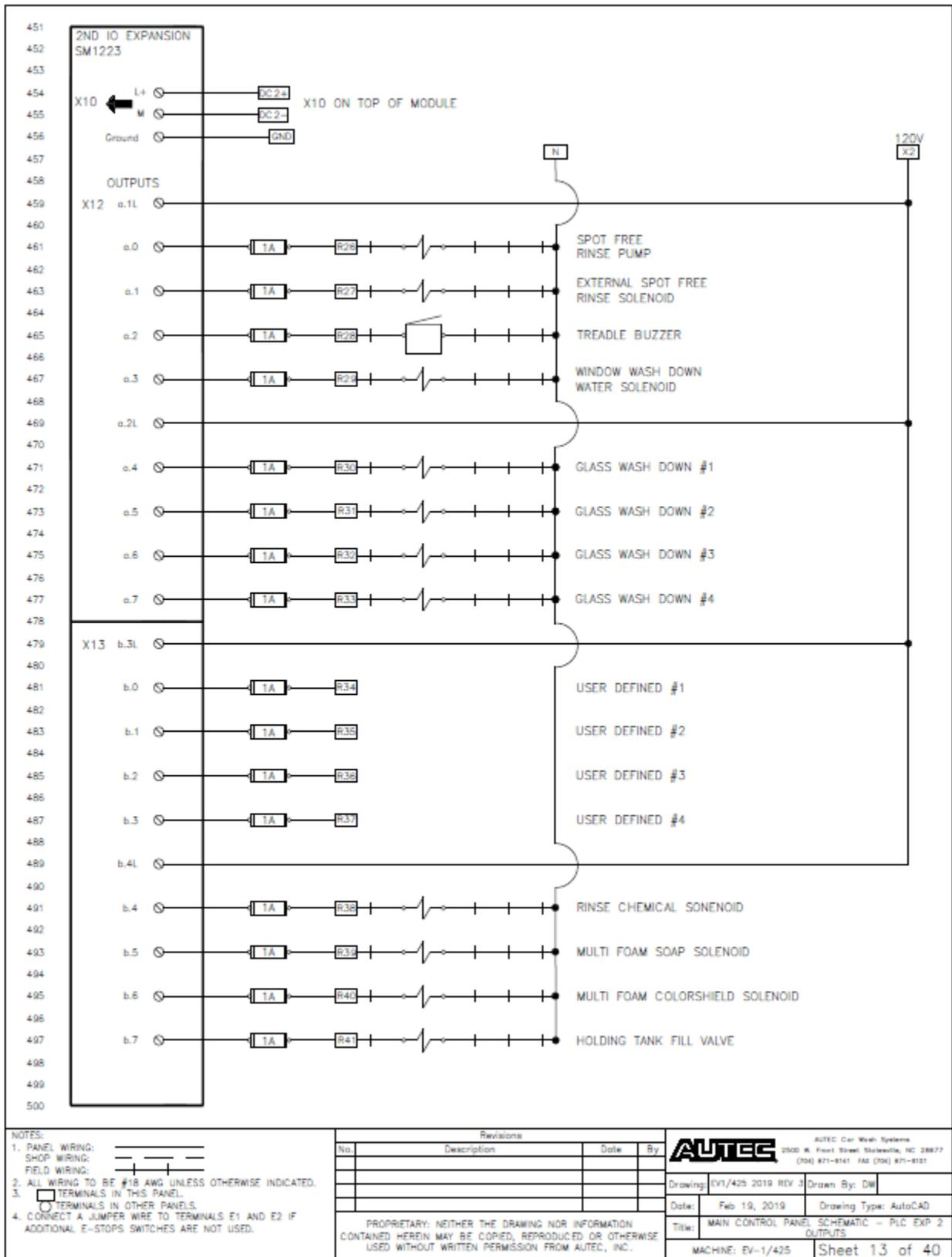
Fig 9-13 Main Control Panel Schematic – Mod 2 Outputs
