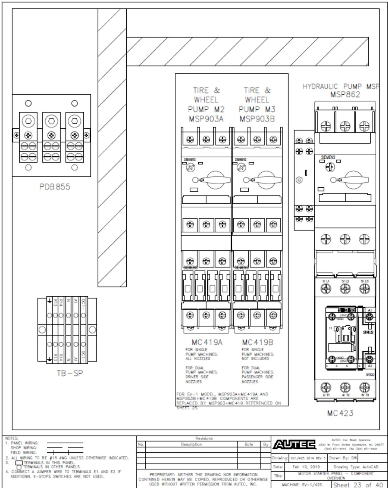
Fig 9-23 Motor Starter Panel – Component Overview
