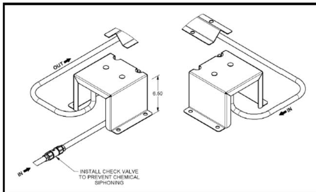
3. Assemble barbs on check valve and position it inline near the Primary unit.
