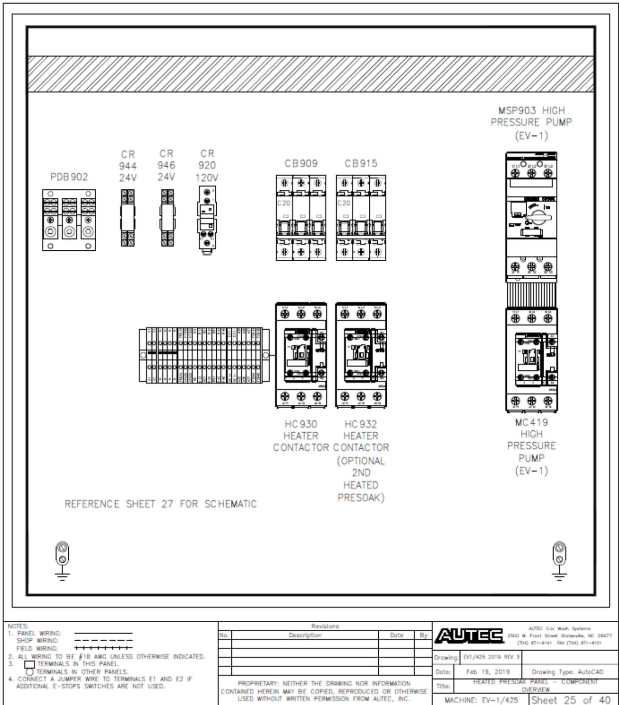
Fig 9-25 Heated Presoak Panel – Component Overview
