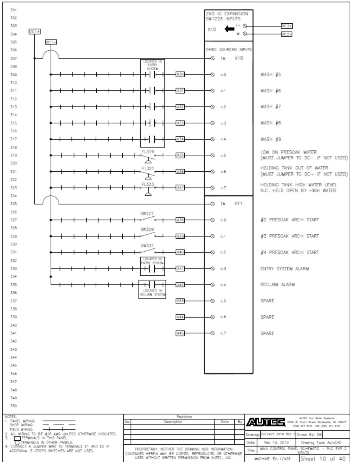
Fig 9-10 Main Control Panel Schematic – Mod 2 Inputs
