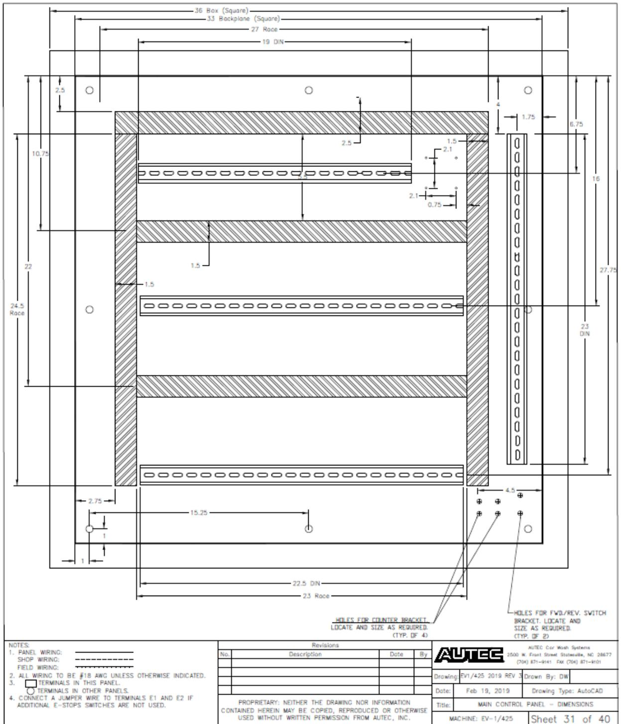
Fig 9-31 Main Control Panel – Dimensions
