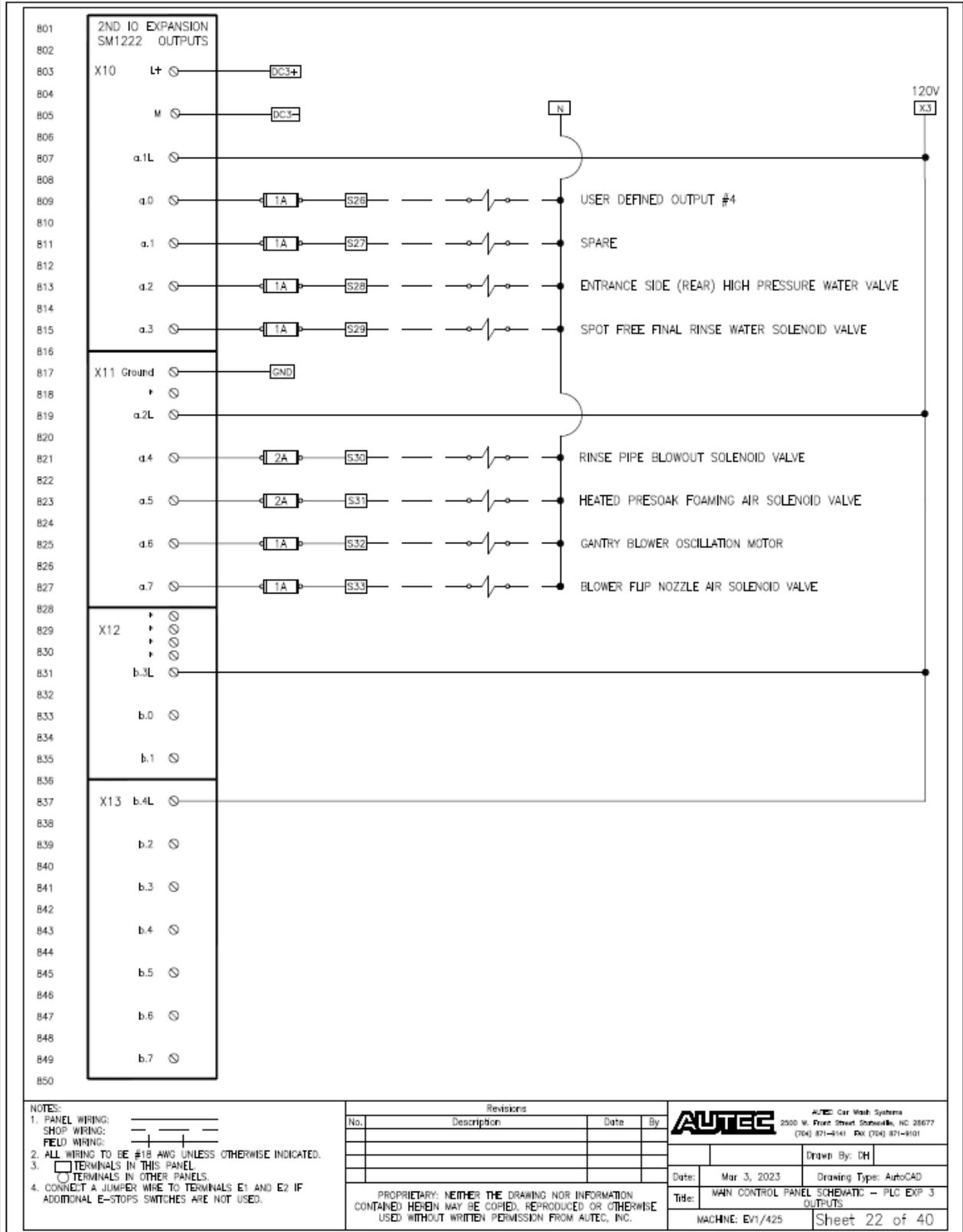
Fig 9-22 Gantry Control Panel Schematic – Mod 2 Outputs
