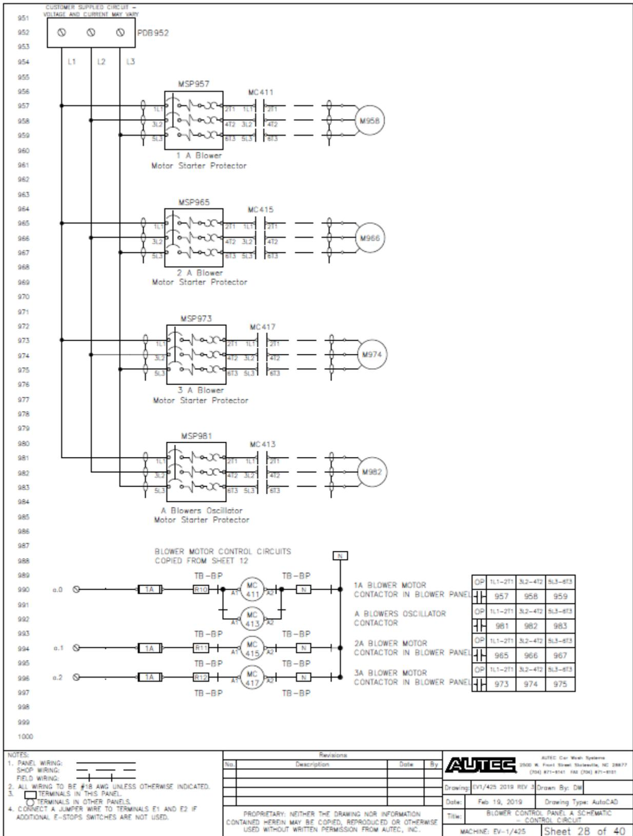
Fig 9-28 Blower Control Panel A Schematic – Control Circuit
