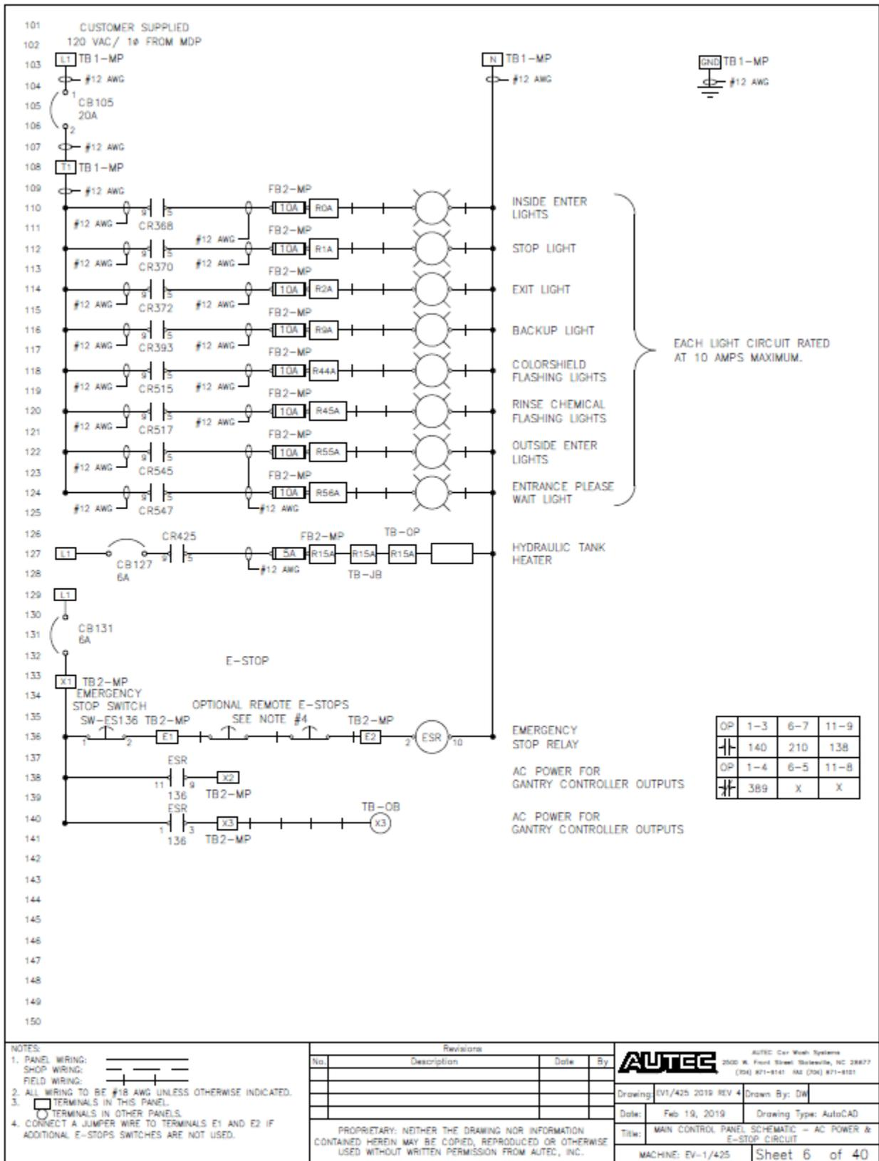
Fig 9-6 Main Control Panel Schematic – AC Power & E-Stop
