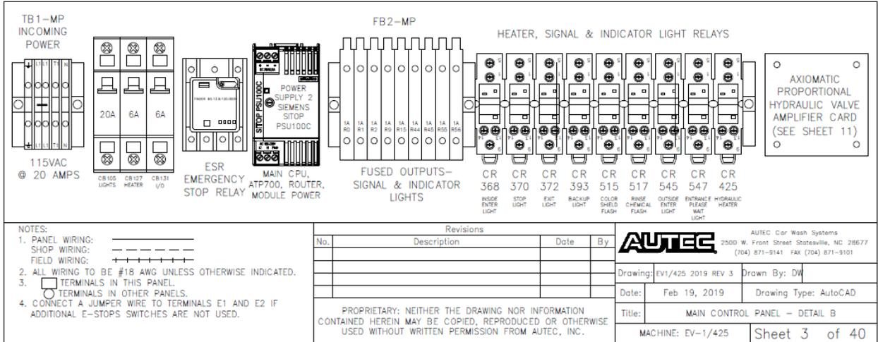
Fig 9-3 Main Control Panel – Detail B
