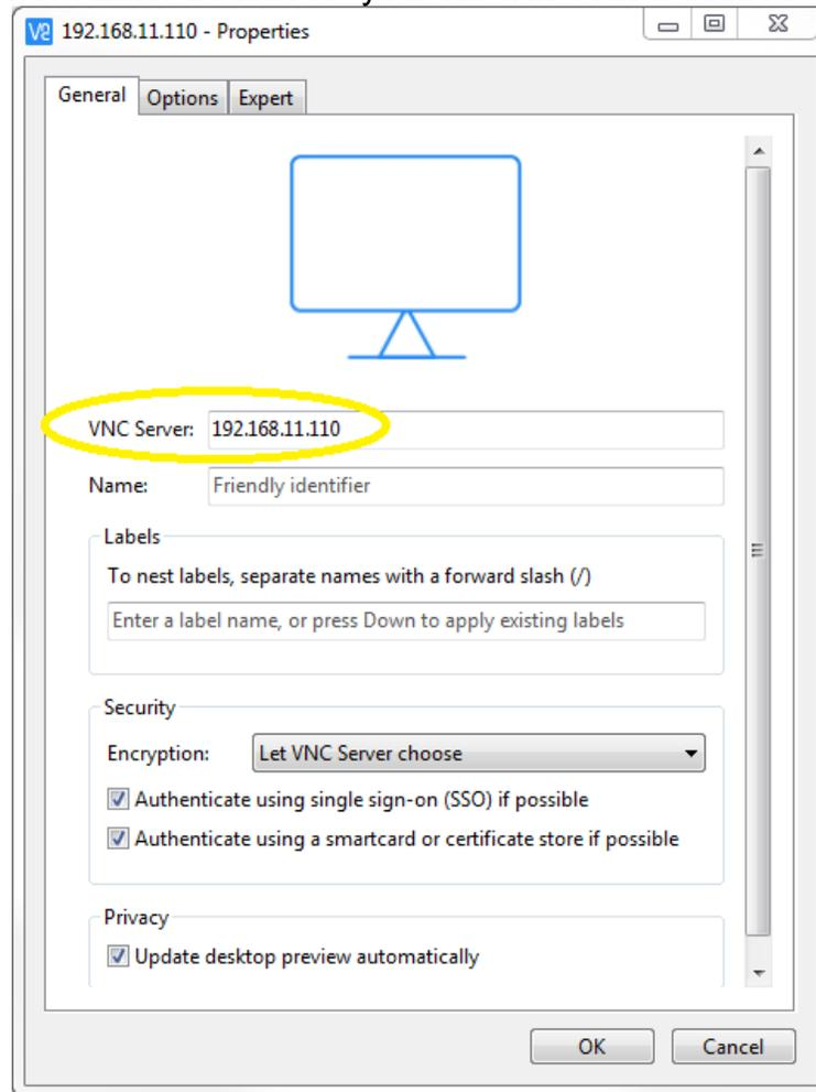
Figure 7-47 Enter IP address in VNC Viewer
