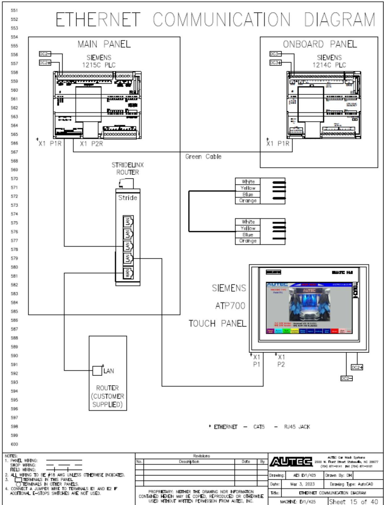
Fig 9-15 Ethernet Communication Diagram
