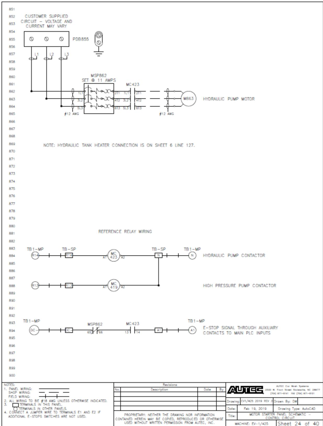
Fig 9-24 Motor Starter Panel Schematic – Control Circuit
