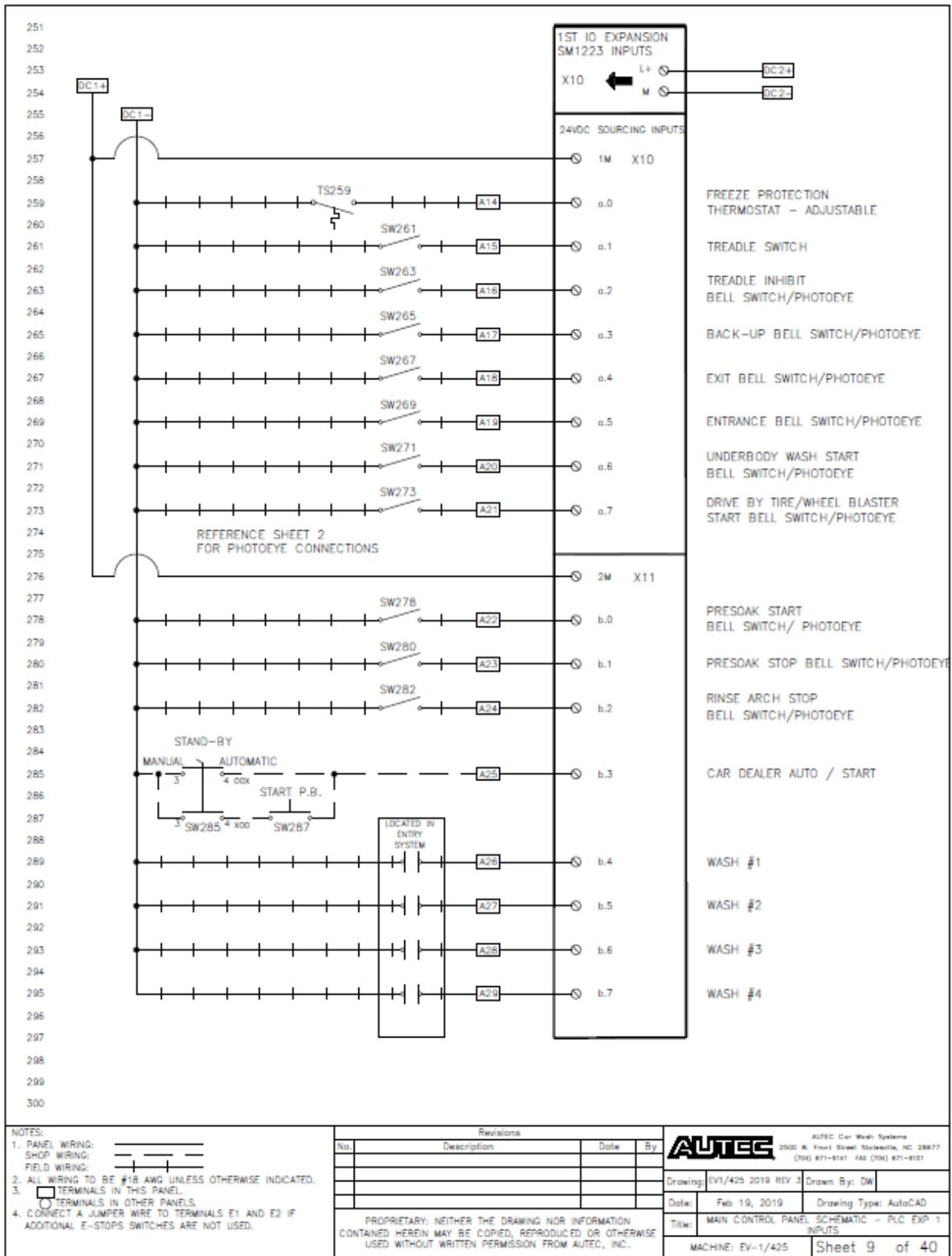
Fig 9-9 Main Control Panel Schematic – Mod 1 Inputs
