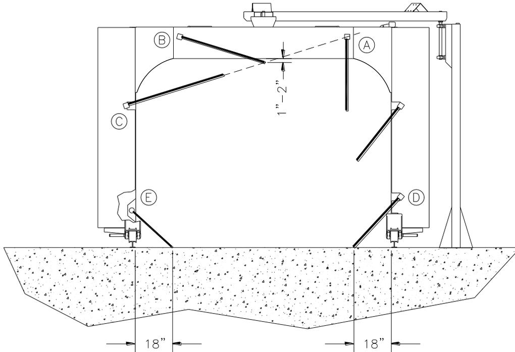
A. Top header nozzles - At the maximum oscillator down stroke the top nozzles should point straight down.
