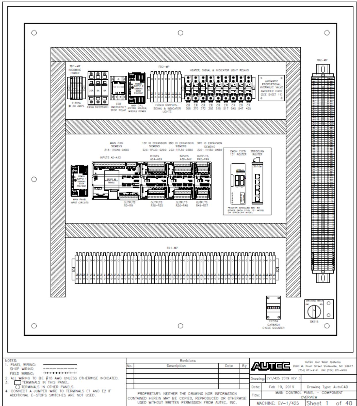
Fig 9-1 Main Control Panel – Component Overview
