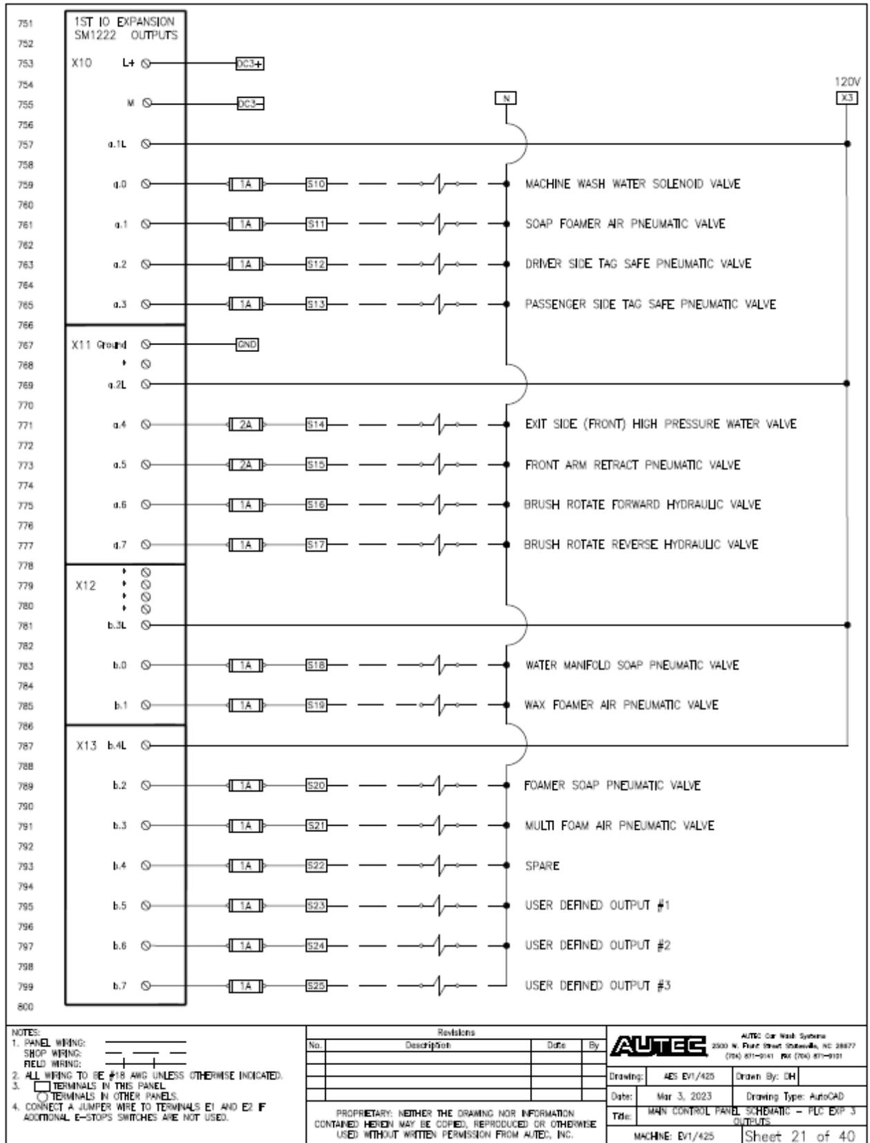
Fig 9-21 Gantry Control Panel Schematic – Mod 1 Outputs
