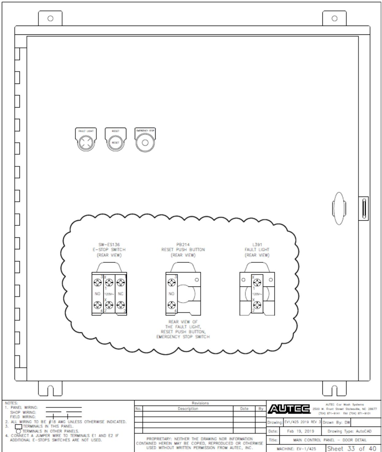
Fig 9-33 Main Control Panel – Door Detail
