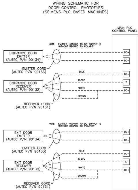
Photoeyes are to be wired normally closed, light operate (receiver output conducts when the light beam is clear). This schematic is for Banner SM30 Series, 24VDC photoeyes. For other photoeyes, refer to the manufacturer's instructions for proper installation.
