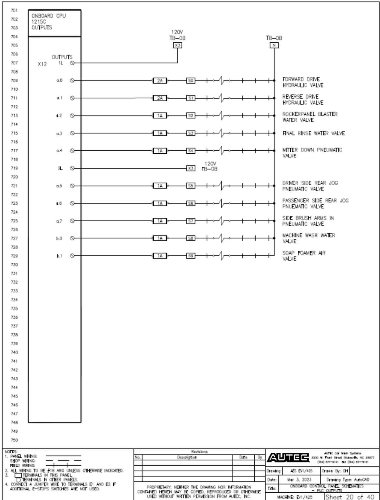
Fig 9-20 Gantry Control Panel Schematic – PLC Outputs
