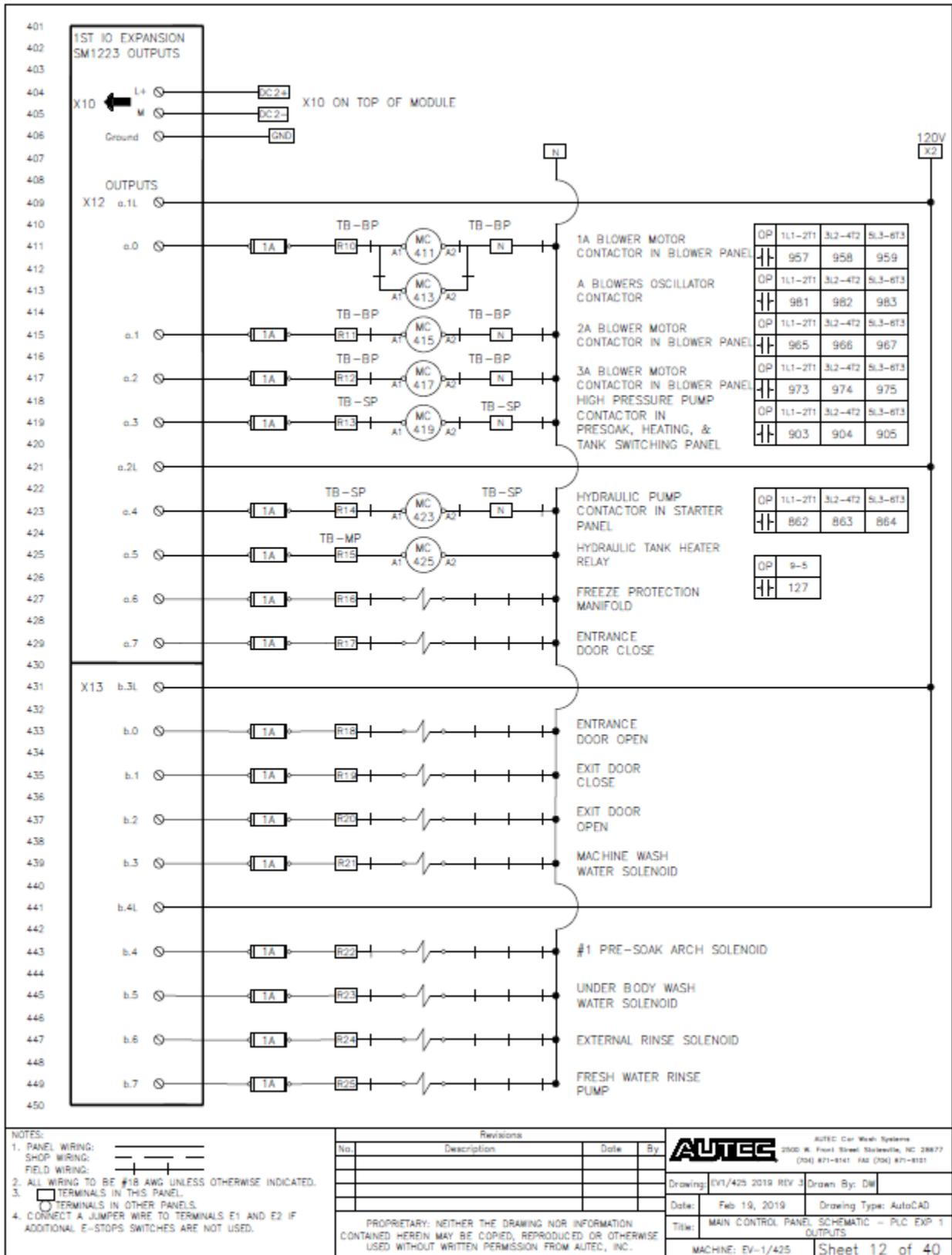
Fig 9-12 Main Control Panel Schematic – Mod 1 Outputs
