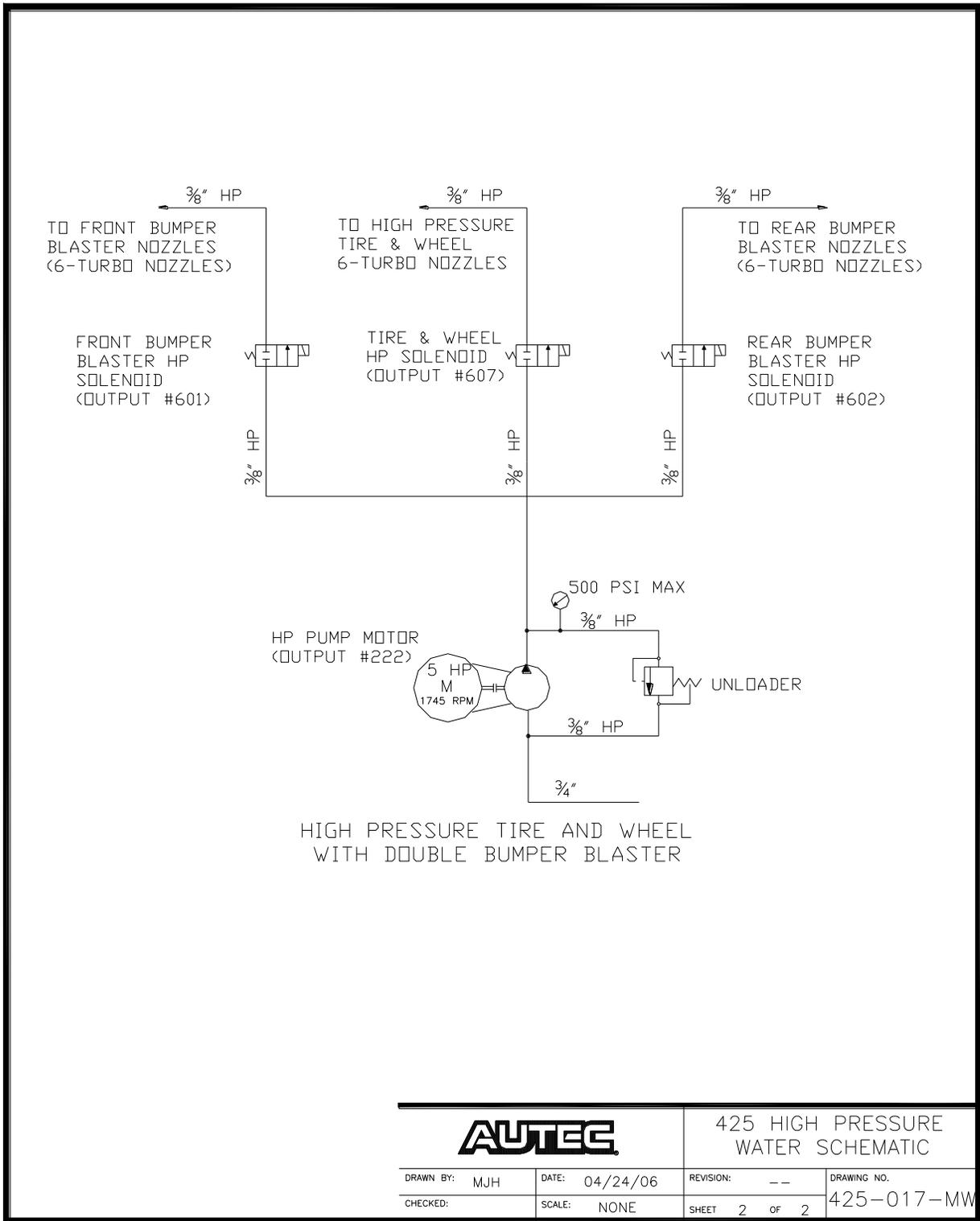
Fig 10-10 High Pressure Pumping Station (Optional)
