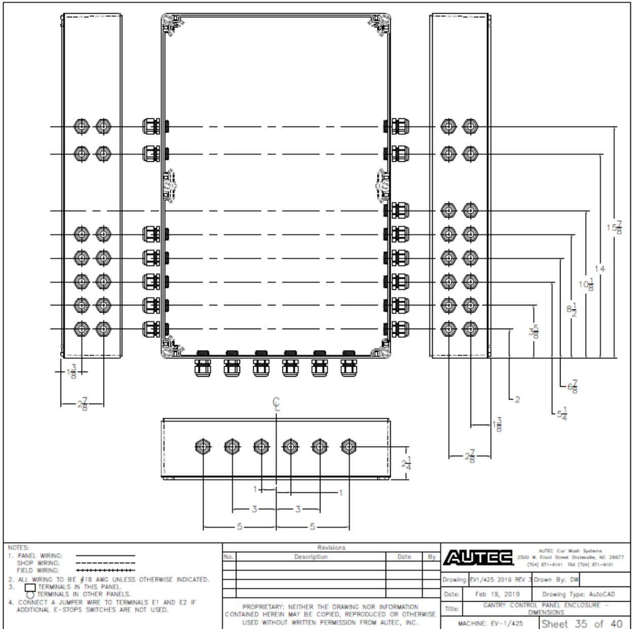
Fig 9-35 Gantry Control Enclosure – Dimensions
