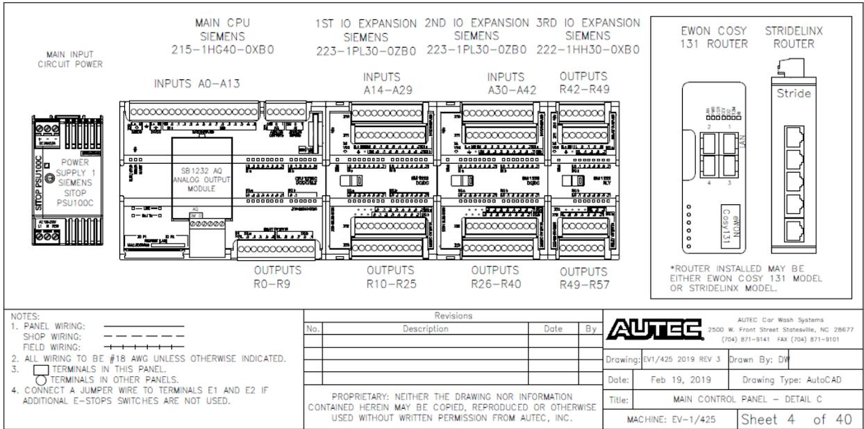
Fig 9-4 Main Control Panel – Detail C
