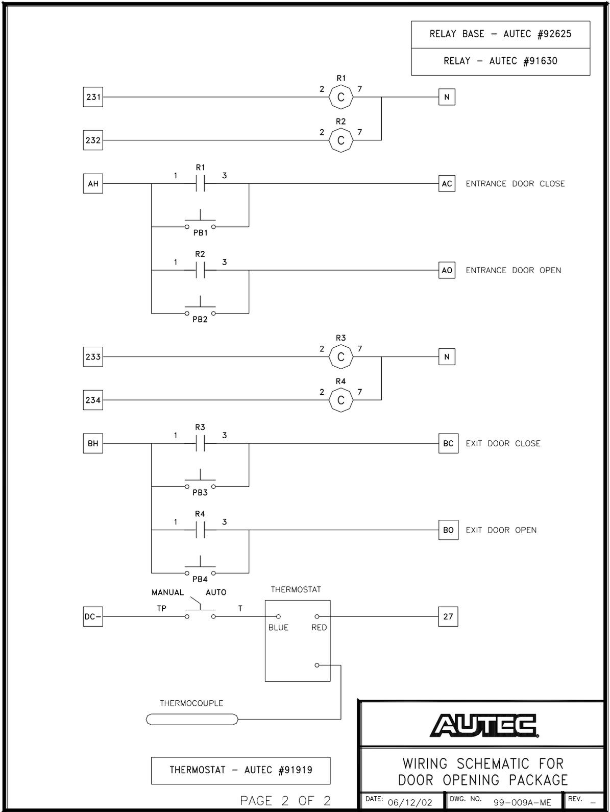
Fig 13-3 Wiring Schematic for Optional Door Control Package
