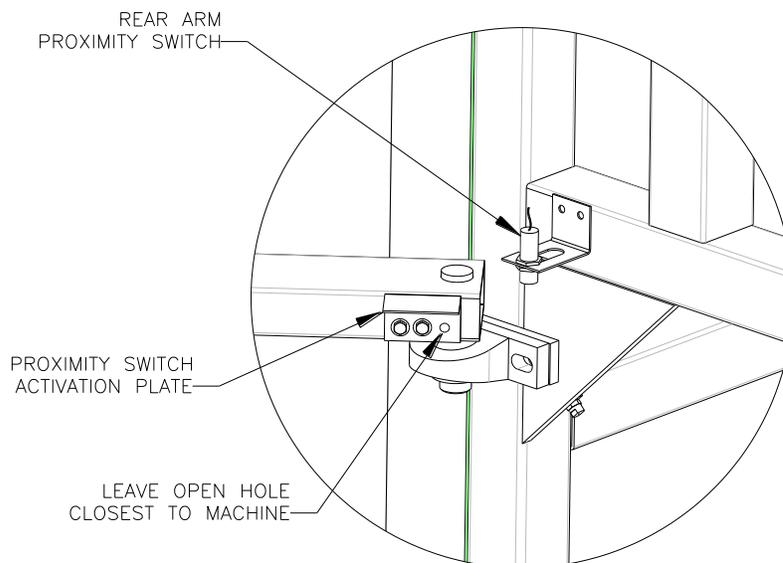
Figure C – Rear Arm Proximity Switch Installation
