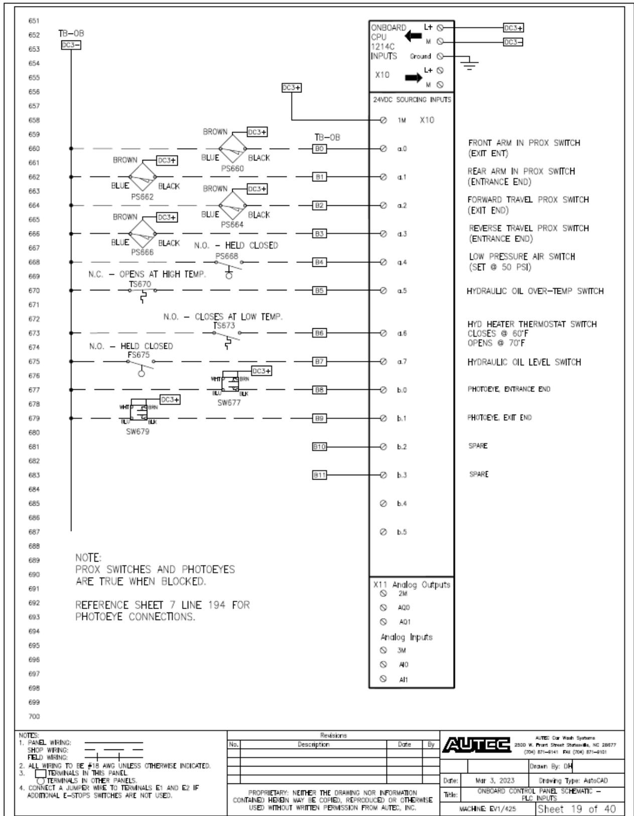
Fig 9-19 Gantry Control Panel Schematic – PLC Inputs
