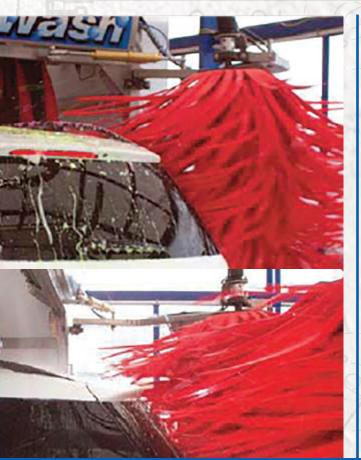
Arms are inclined towards the vehicle to better fit the vehicle contour
