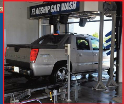
Flagship's wash process is completed by 'super dry-blow dry' high velocity blowers
